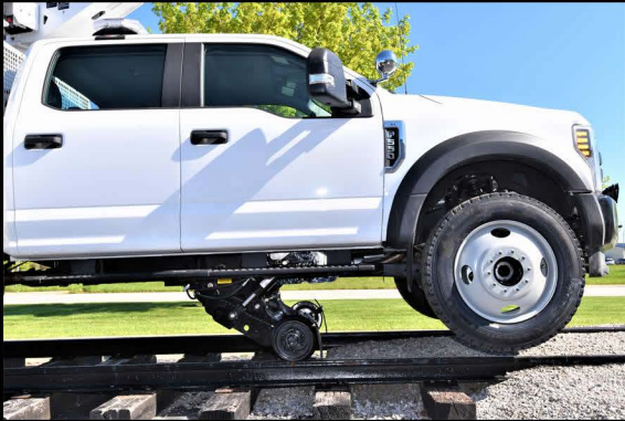
Front Under-Cab Rail Gear
